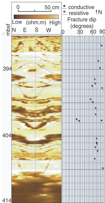
**Figure 4.** Static normalised RAB image of the frontal thrust zone. The unwrapped  $360^\circ$  image shows planar dipping fractures as sinusoids whose attitude is shown to the right of the image. Most fractures are conductive (dark) but the zone is resistive (light).
