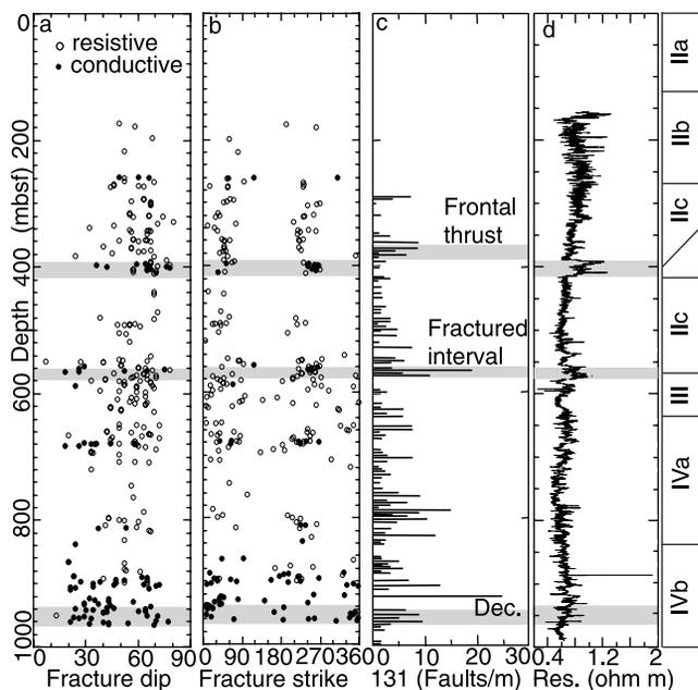
**Figure 2.** Interpreted 808 fractures from RAB images (a, b - strike as right hand rule) and Leg 131 cores (c). Resistive (open circles) and conductive (filled circles) fractures are indicated. Three major deformation zones are recognised: 1) frontal thrust zone; 2) fractured interval; and 3) décollement (Dec.). (d) Leg 196 resistivity data. Lithologic facies to right, [Taira *et al.*, 1991]. IIa, b U. and L. Axial trench; IIc Trench wedge; III Trench to basin; IVa, b U. and L. Shikoku basin.
