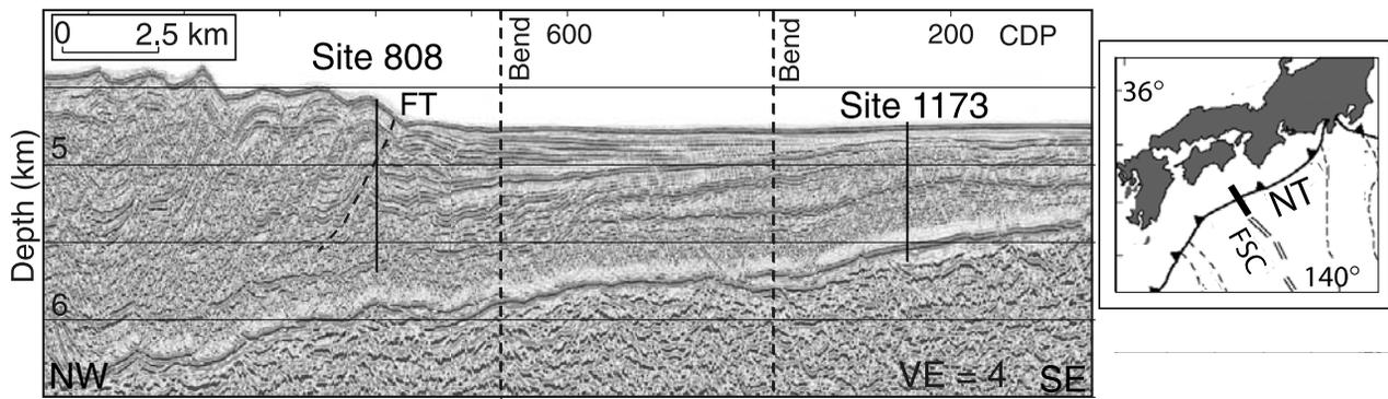
**Figure 1.** Seismic profile across Leg 196 sites [Mikada *et al.*, 2002]. Nankai Trough (NT) setting, line indicates profile. FSC = Fossil Spreading Centre; FT = frontal thrust.
