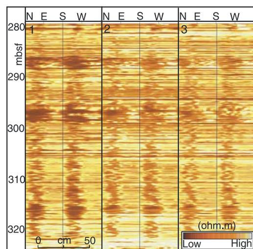
**Figure 5.** Static normalised RAB image within Unit 2. Borehole breakouts are two dark lines  $180^\circ$  apart representing borehole elongation in the direction NE-SW ( $\sigma_2$ ). Three images represent resistivity 1" (1), 3" (2) and 5" (3) from borehole. Deformation decreases away from the borehole.
