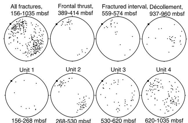
**Figure 3.** Equal area projections of poles to fracture planes at Site 808 from RAB images, square = convergence vector. The three main deformation zones and all fractures are shown. Second row shows fracture orientations within each log unit with fractures of the three main fault zones removed.
